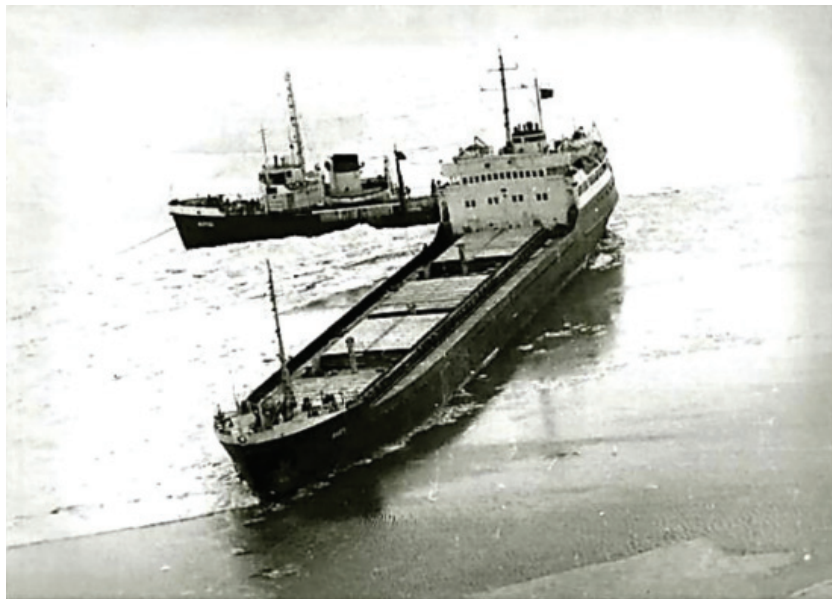
Figure 7. Bulk Carrier MV Baku on seabed and SDT attempting to unground the vessel. Photo by Bukharitsin P.I. 1981
