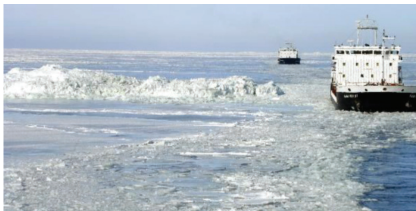
Figure 3. Illustration of ridged grounded features forming in vicinity of Volga-Caspian channel. (Bukharitsin, 2011)
