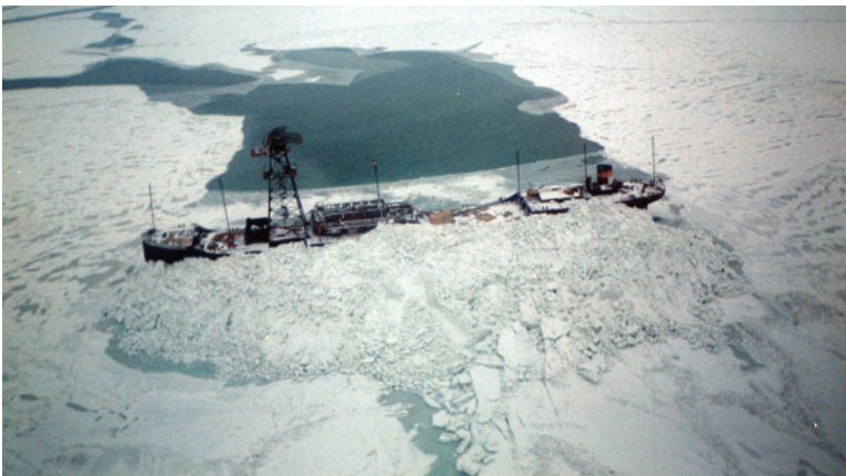
Figure 4. At the lee face of stranded ice, as a rule, area of clear water is formed – ice-holes and canals
