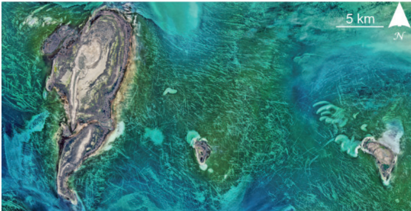
Figure 21. Ice scours on the Northern Caspian Sea bottom, Tyuleniy Archipelago (acquired 16 April 2016) [61]
